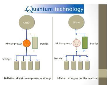
Schematic of Quantum Recovery and Purification System for LTAs.
